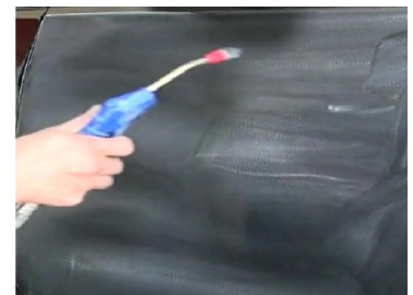
c) Air blowing, after TOLEX sanding And Defects can be visible.
